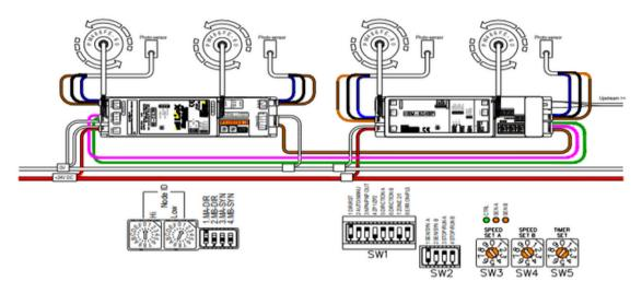
An HBM-604B can exchange handshake signals with the IB-E03B and IB-E04F. Product will accumulate at the last zone before the IB card. When sensor A is blocked on the HBM-604B, it sends the sensor out signal to the IB. The IB then sends a force run signal to the HBM. If an HBM-604B has an error, the error output signal is pulsed from the HBM-604B to the IB card which can determine the error condition and bring it to upper level Ethernet communication.
